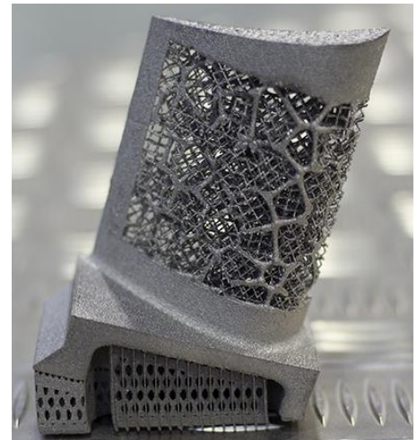
Figure 1 An example of a additively manufactured Meta-crystal, which contains different lattice structures to achieve best mechanical properties
